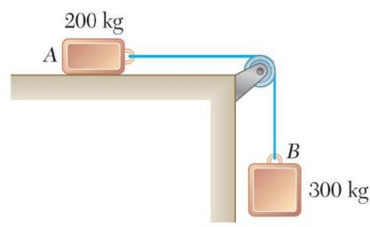
Two blocks are joined by an inextensible cable as shown. If the system is released from rest, determine the velocity of block *A* after it has moved 2 m. Assume that the coefficient of friction between block *A* and the plane is  $\mu_k = 0.25$  and that the pulley is weightless and frictionless.
