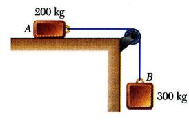
• When the two relations are combined, the work of the cable forces cancel. Solve for the velocity.
