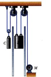
The dumbwaiter D and its load have a combined weight of 600 lb, while the counterweight C weighs 800 lb.
