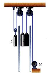
• In the first case, bodies are in uniform motion. Determine force exerted by motor cable from conditions for static equilibrium.
