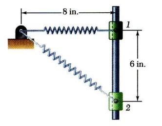
A 20 lb collar slides without friction along a vertical rod as shown. The spring attached to the collar has an undeflected length of 4 in. and a constant of 3 lb/in.
