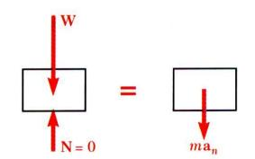
• Apply Newton's second law to find minimum radius of curvature at point 3 such that a positive normal force is exerted by the track.
