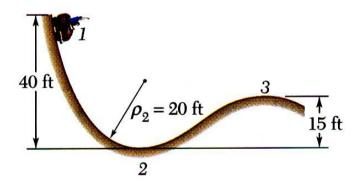
A 2000 lb car starts from rest at point 1 and moves without friction down the track shown.
