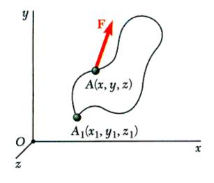
• Concept of potential energy can be applied if the work of the force is independent of the path followed by its point of application.
