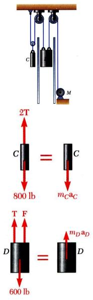
• In the second case, both bodies are accelerating. Apply Newton's second law to each body to determine the required motor cable force.
