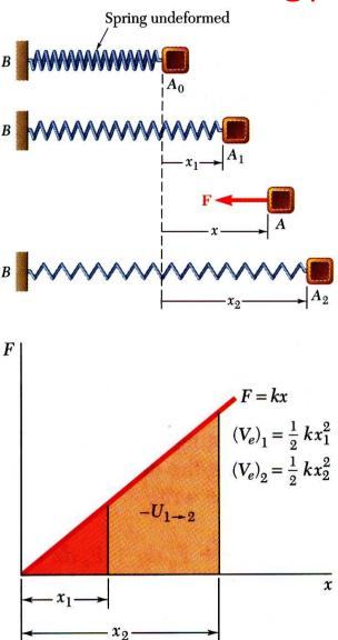
• Work of the force exerted by a spring depends only on the initial and final deflections of the spring,
