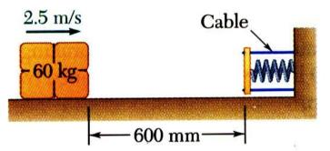
A spring is used to stop a 60 kg package which is sliding on a horizontal surface. The spring has a constant k = 20 kN/m and is held by cables so that it is initially compressed 120 mm. The package has a velocity of 2.5 m/s in the position shown and the maximum deflection of the spring is 40 mm.
