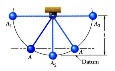
$T_1 = 0 \quad V_1 = W\ell$  $T_1 + V_1 = W\ell$
